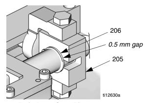
Fig. 29: Ratio Beam Snap Ring
